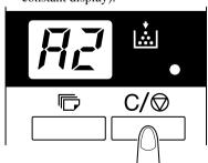
While the pause function is enabled, it is possible to exit the Cycle Print Mode by pressing the Clear key a second time (the value displayed in the "No. of Copies" display will change to a "1".)
